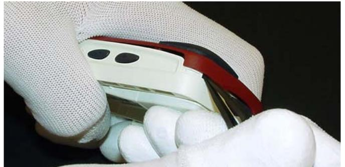
The A-Cover can be released from the lower right side on. Place the plastic tweezers between the cover clip and the power button. Same has to be done at the left side just near the Port Cover.
