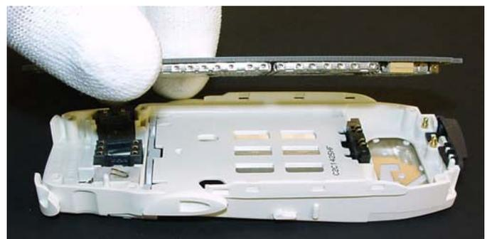
Now you can lift up the CMT module MA4 from the D-Cover. The Buzzer, SIM Card Reader, Vibra, Battery Connector, Pogo Pins, Power Button and the Battery Lock are only squeezed into the D-Cover and can be changed easily.
